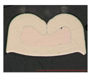
Figure V-5: Micro-section of a flawless sample
