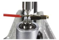
Figure V-11: Detail view of a crimp contact between the measuring tips
