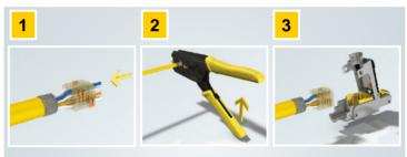
Cable preparation and insertion of the individual wire cores according to the wiring diagram used for the preLink® terminal module.
