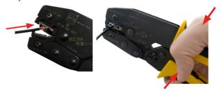
3. Remove the crimped contact.
