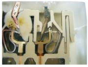
Figure VI-7: The consequences of improper assembly (shown here on the Han® ES), close-up
