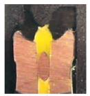
Figure XI-23: Contact with a solid wire core
