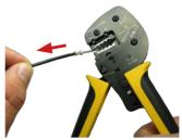
3. Upon relase, the handles will open automatically and the crimped contact can be removed
