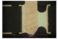
Figure IX-10: Soldered joint with marginal fill level
