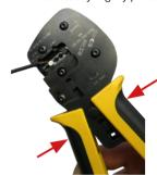
2. Crimp both components by closing the handles until the controlled accessories cycle mechanism releases.
