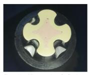
Figure V-1: Micro-section of a flawless sample
