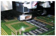
Figure IX-5: Pick-and-place machine with vacuum pipette and D-Sub
